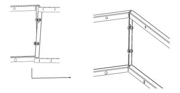
When all parts are put together then gently turn the collar in the right direction. Control that the edge bends are at the same level.
